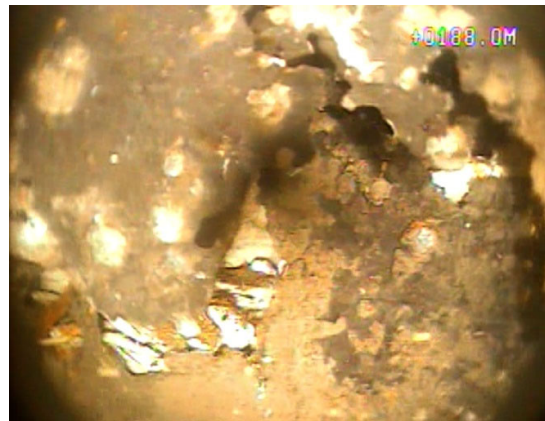
Large hole noted through mild steel casing wall at 188.00m.
