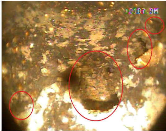
Large hole noted through mild steel casing wall at 187.90m.
