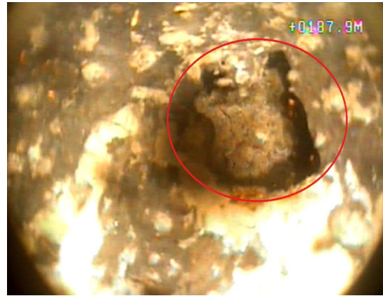
Large hole noted through mild steel casing wall at 187.90m.
